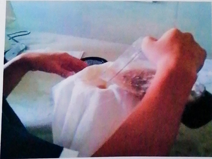
Plate 2. The slurry is filtered through a triple layered cheesecloth to a beaker after blending with distilled water.
