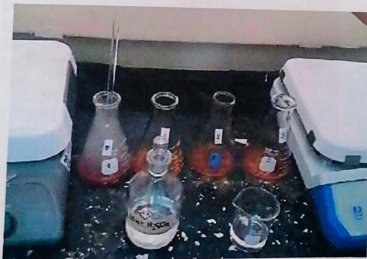
Plate 14. The addition of a strong acid \text{H}_2\text{SO}_4 to the Potassium dichromate solution will bring about hazardous fumes thus it was conducted within a fume hood.
