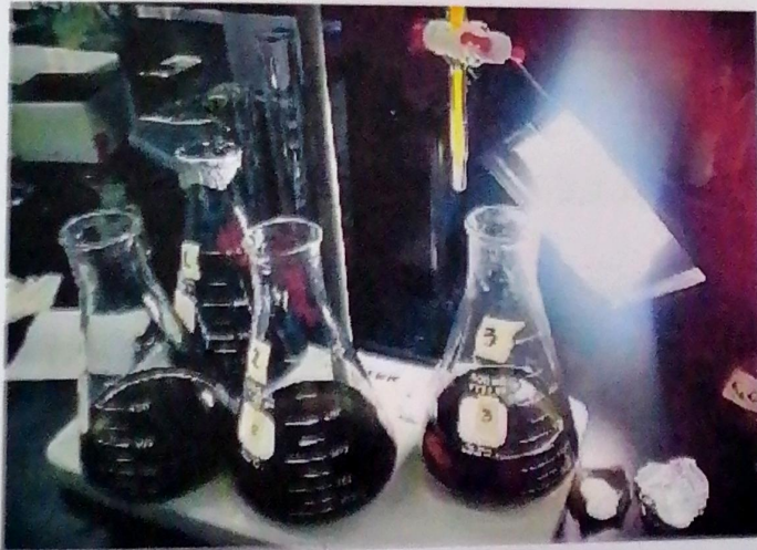
Plate 16. After each titration during every few milliliters of interval it is compared ensure the end point and the titer values were then recorded.
