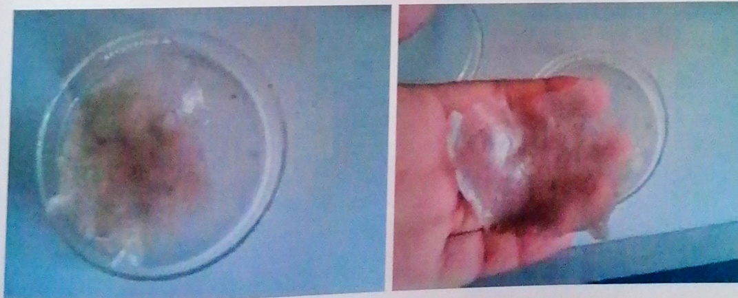
Plates 6-7. After oven drying for 2 hours at 65^{\circ}\text{C} , the final product of the produced bioplastic film had a smooth feel and a light grayish to opaque in visualization of color. It was quite thick and strong by manual testing.
