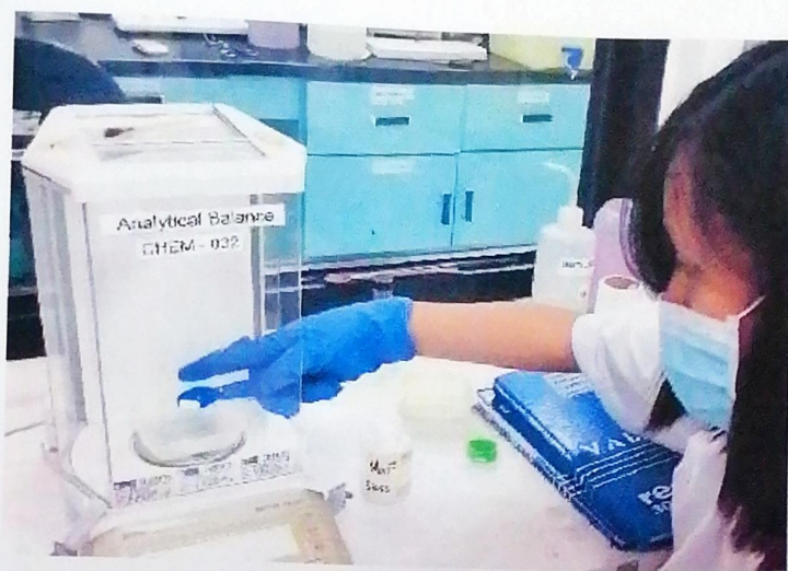
Plate 8. An exact amount of 1 gram sodium fluoride( \text{NaF} ) was weighed using a closet-type analytical balance at the DOST chemical laboratory.
