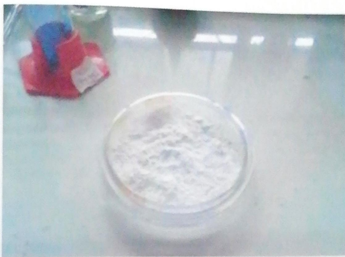
Plate 3. The remaining starch granules are left to air dry overnight at room temperature then stored in a petri dish until intended use and the extraction process was repeated numerous times.
