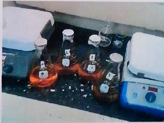
Plates 11-12. One normal potassium dichromate ( K_2Cr_2O_7 ) is diluted in deionized water. It is carcinogenic chemical, thus it is diluted and transferred to individual flasks handled with caution.
