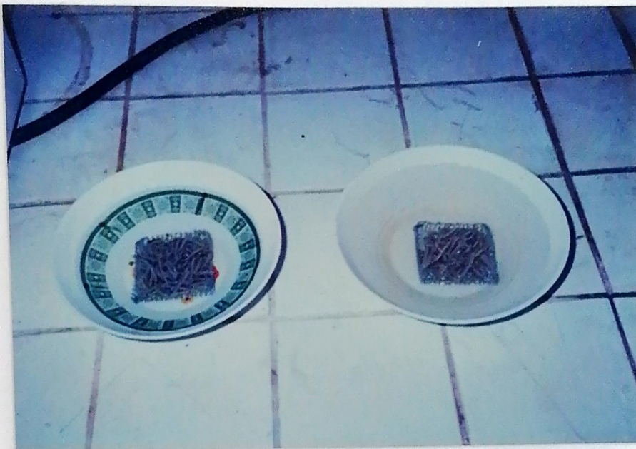
Plate No. 5 The samples are being submerged in bowls filled with tap water for water stability test.
