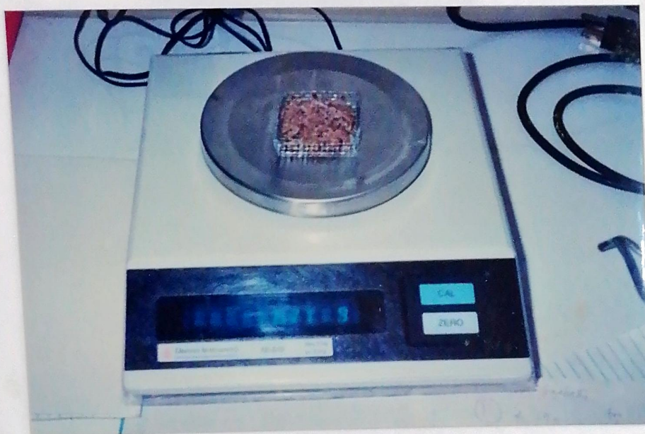
Plate No. 8 A sample is being weighed using an analytical balance for the final procedure in the water stability test.
