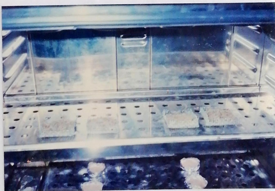
Plate No. 6 After 10 minutes of submersion, the samples are being dried in the oven for four hours.
