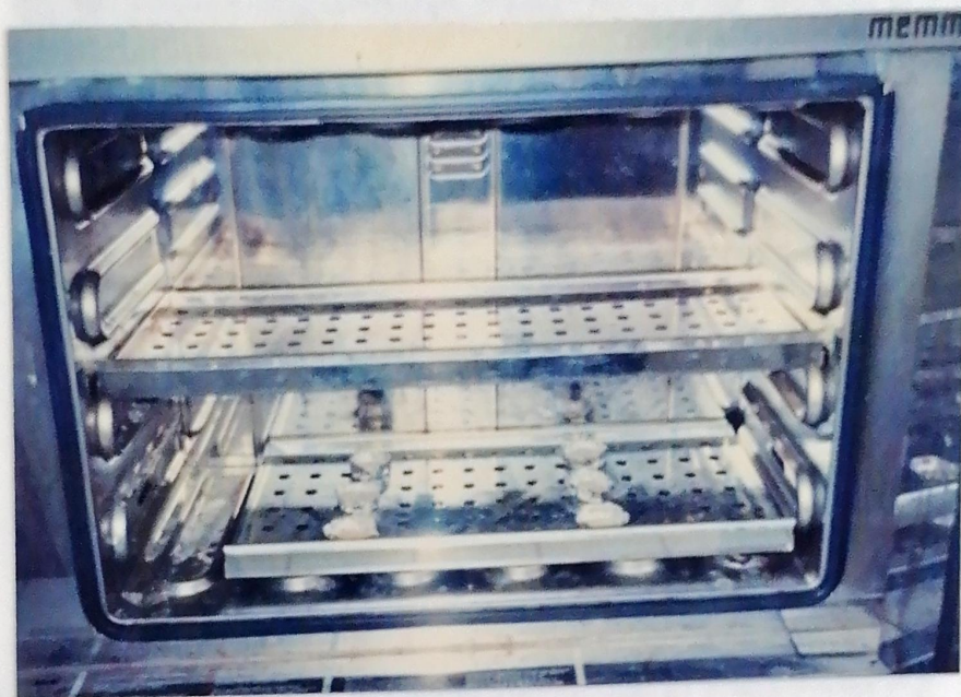
Plate No. 3 The feed samples for moisture determination test are being oven-dried for six hours.
