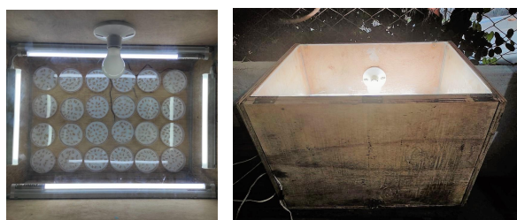
Figure 1. Incubator setup. Left: top view, with petri dishes containing RC222 seeds. Right: front view.
