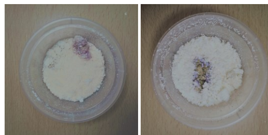
Figure 1. Crude cellulose extracted via CM (left) and MAM (right) were tested for analyte validity using Schultze's reagent, to which the purplish color indicated the presence of cellulose.
