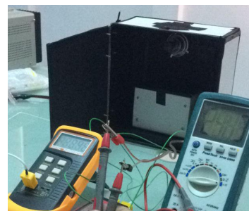
Figure 1. Photo of the setup with the PV cell, PCM inside the aluminum container, xenon lamp inside a dark box, multimeter for the measuring of the voltage and k-type thermocouple thermometer for measuring the temperatures.
