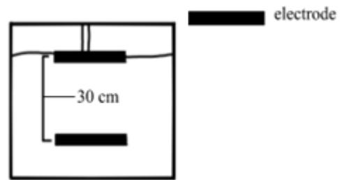
Fig. 2: Individual P-MFC Setup. The lower electrode is the anode.
