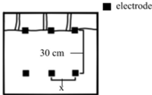
Fig. 3: Shared-anolyte P-MFC. The x represents the plant spacing for the different setups which are 5, 7, 9 cm.
