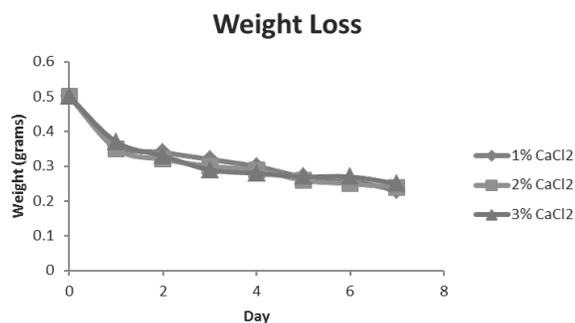
Fig. 3: Weight loss of slow-release beads for seven days.
