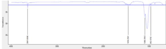
Fig. 2: Infrared spectra of extracted hydroxyapatite
