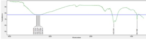
Fig. 1: Infrared spectra of extracted chitosan
