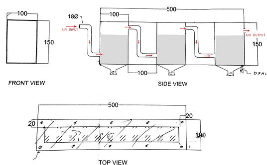
Fig. 2: Interior of the proposed design of T.E.R.R.A.
