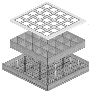
Fig. 3: Assembly of Cover Lids, Storage Units and Web Collectors
