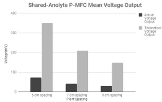
Fig. 4: Shared-anolyte P-MFC Mean Voltage Output
