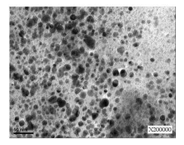
Fig. 4: Transmission electron microscope image of AgNPs synthesized with 15-g *Moringa oleifera sp.* seed extract.
