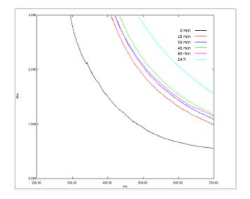
Fig. 3: Absorbance level of AgNPs solution using 15-g *Moringa* oleifera sp. seed extract.
