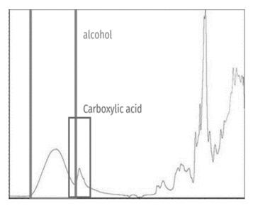
Fig. 5: Functional groups present in the cellophane spectra. The peaks in the cellophane sheet indicate the presence of functional groups, such as alcohol and carboxylic acid.
